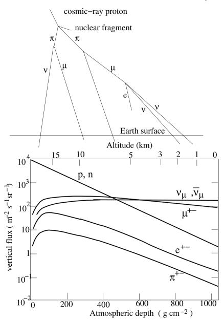
**Fig. 5.4.** An example of a "shower" induced by a cosmic-ray proton in the upper atmosphere. Two pions and a nuclear fragment are produced when the proton strikes a nucleus. The two pions decay  $\pi \to \mu \nu$ . and one of the muons decay  $\mu \to e \nu \bar{\nu}$  The undecayed muon reaches the Earth's surface where it stops because of ionization energy loss. The lower panel shows the fluxes as a function of depth in the atmosphere [54].
