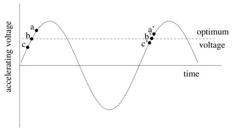
Fig. B.4. The principle of phase stability in a linear accelerator. Particles arriving in a gap at point b are accelerated such that they arrive at the text gap at the point b' with the same phase with respect to the alternating field. Particles arriving at point a (c) receive more (less) acceleration and therefore arrive relatively earlier (later) in the next gap, point a' (c'). Particles in the range a-c are thus "focused" in phase-space toward the point b.
