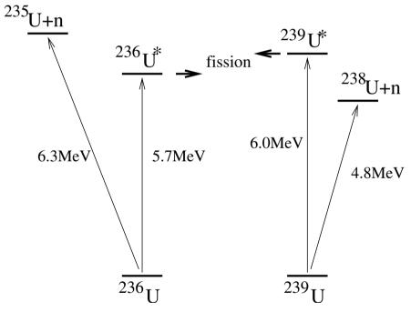
**Fig. 6.6.** Levels of the systems A=236 and A=239 involved in the fission of  $^{236}\mathrm{U}$  and  $^{239}\mathrm{U}$ . The addition of a motionless (or thermal) neutron to  $^{235}\mathrm{U}$  can lead to the fission of  $^{236}\mathrm{U}$ . On the other hand, fission of  $^{239}\mathrm{U}$  requires the addition of a neutron of kinetic energy  $T_{\rm n}=6.0-4.8=1.2\,\mathrm{MeV}$ .
