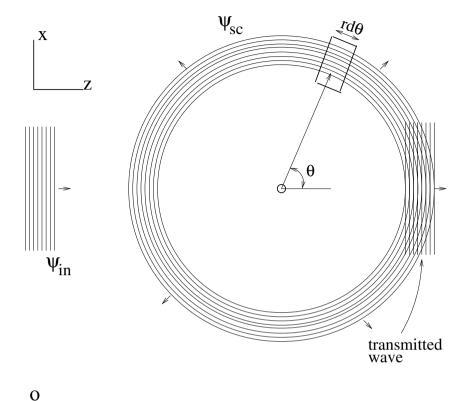
Fig. 3.14. A wave packet that impinges upon a region with  $V(r) \neq 0$  will interact in a way that will produce a scattered wave packet and a transmitted wave packet. The probability to find the particle in the box in the scattered wave is proportional to the differential scattering cross-section,  $d\sigma/d\Omega$ .
