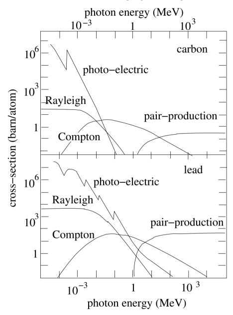
Fig. 5.12. Photon cross-sections on carbon and lead [1] as explained in the text. At low energy,  $1 \,\mathrm{keV} < E < 100 \,\mathrm{keV}$ , photo-electric absorption dominates while electron–positron pair production dominates for  $E \gg 2 m_\mathrm{e} c^2$ . Compton scattering dominates at intermediate energies. Photo-nuclear absorption (Fig. 3.8) is of minor importance.
