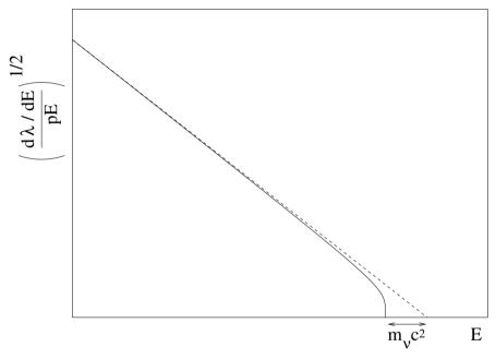
Fig. 4.17. The Kurie plot near the electron maximum energy in the case of  $m_{\rm v}=0$  (dashed line) and  $m_{\rm v}\neq 0$  (solid line).
