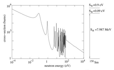
Fig. 6.17. The radiative neutron capture cross-section on  $^{149}$ Sm. The absorption resonances correspond to excited states of  $^{150}$ Sm that are above the neutron-separation energy  $S_{\rm n}=7.987\,{\rm MeV}$ . The diagram on the right shows the ground state and the first two states responsible for the resonances. The first one at  $S_{\rm n}+0.09$  can resonantly absorb thermal neutrons ( $3kT=0.078\,{\rm eV}$  for  $T=300\,{\rm K}$ ).
