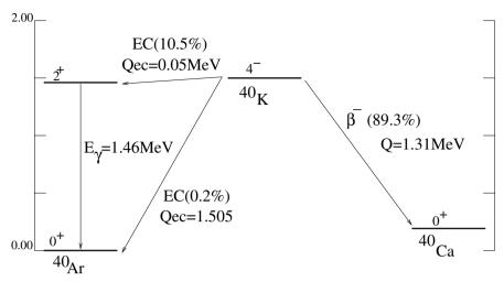
**Fig. 5.1.** The β-decay of  $^{40}$ K. Being an N-odd,Z-odd nucleus, it has two modes: electron capture to  $^{40}$ Ar and β $^-$  to  $^{40}$ Ca. The long half life (1.28×10 $^9$ yr) is explained by the large angular momentum changes in the decays to the ground states (making the decays highly forbidden) and the small value of  $Q_{\rm ec}$  to the  $2^+$  state of  $^{40}$ Ar.
