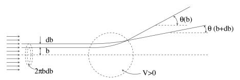
Fig. 3.9. The scattering of a particle of momentum p by a repulsive force. The trajectories for impact parameters b and b+db are shown. The probability that a particle is scattered by an angle between  $\theta(b)$  and  $\theta(b+db)$  is proportional to the surface area  $2\pi b db$ .
