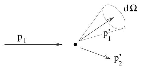
Fig. 3.17. Scattering of two particles with recoil.
