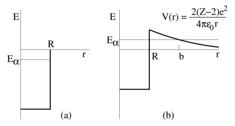
Fig. 2.16. Gamow's model of  $\alpha$ -decay in which the nucleus contains a  $\alpha$ -particle moving in a mean potential. If the electromagnetic interactions are "turned off", the  $\alpha$ -particle is in the state shown on the left. When the electromagnetic interaction is turned on, the energy of the  $\alpha$ -particle is raised to a position where it can tunnel out of the nucleus.
