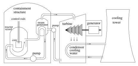
Fig. 6.10. Schematic of a pressurized water reactor.
