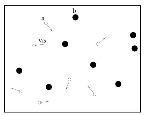
Fig. 3.3. A box containing two types of particles, a and b. The a particles move in random directions with velocity  $v_{ab}$  and can interact with the b particles (at rest) to form particles c and d with cross-section  $\sigma_{ab\to cd}$ . The time rate of change of the number density of particles a is determined by the Boltzmann equation (3.31).
