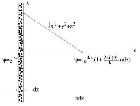
Fig. 3.28. A plane wave,  $\psi = \exp(ikz)$  is incident from the left on a thin slice of material of thickness dz containing a density n of scatterers. Beyond the slice, the wave is the sum of the incident wave and the scattered waves from all scatterers in the slice. As shown in the text, the wavefunction takes the form of Equation (3.222).
