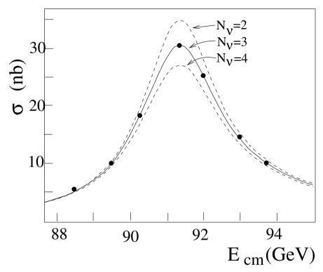
**Fig. 4.31.** Resonance curve of the  $Z^0$  measured by the Aleph experiment at CERN in  $e^+e^-$  collisions at the LEP colliding ring. The three curves represent the theoretical predictions according to the number of different neutrino species. (Courtesy Aleph Collaboration.)
