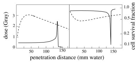
**Fig. 5.15.** Energy loss of ions (left) and survival rate of cells (right) as a function of the penetration depth. Because of the  $v^{-2}$  factor in the Bethe–Bloch formula (5.30), most of the energy is deposited near the stopping point. The dashed curve corresponds to the same quantities for photons. We can see the considerable medical advantage to use heavy ion beams.
