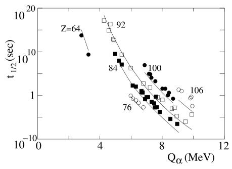
Fig. 2.15. The half-lives vs.  $Q_{\alpha}$  for selected nuclei. The half-lives vary by 23 orders of magnitude while  $Q_{\alpha}$  varies by only a factor of two. The lines shown the prediction of the Gamow formula (2.61).
