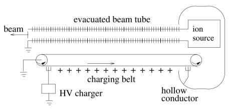
**Fig. B.1.** A schematic of a simple Van de Graff accelerator. Positive charges are transfered from ground potential to a hollow terminal. The ion source is placed inside the terminal and particles are accelerated through the electrostatic field to ground potential.
