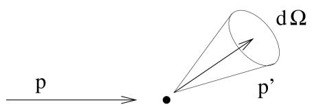
Fig. 3.12. Scattering of a single particle by a fixed potential.
