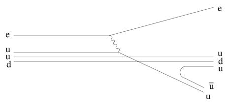
Fig. 3.25. Electron–proton "deep-inelastic scattering." The proton is a bound state und of three quarks. The electron scatters on an individual quark by exchange of a virtual photon. As the quark leaves the proton, a quark–antiquark pair is created. The pair recombines with the initial quarks to make a final state proton (und) and  $\pi^0$  (u $\bar{\rm u}$ ).
