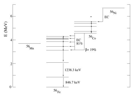
Fig. 8.6. The A=56 system showing the final stage of stellar burning, the  $\beta$ -decays of  $^{56}$ Ni and  $^{56}$ Co.
