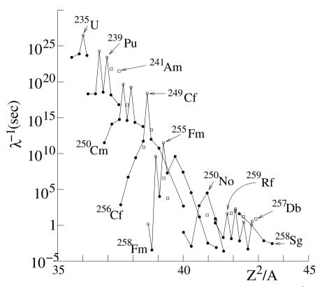
**Fig. 6.4.** Spontaneous fission lifetimes as a function of the fission parameter  $Z^2/A$  for selected nuclei. Circles are for even-Z nuclei, filled circles for even-even nuclei and open circles for even-odd nuclei. Squares are for odd-Z nuclei.
