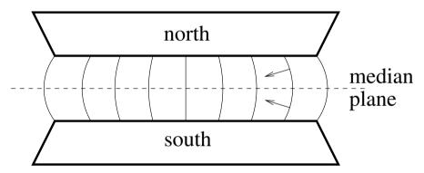
**Fig. B.6.** Vertical focusing in a radially-decreasing dipole magnetic field. Particles in the median plane experience a horizontal force. The force on particles above or below the median plane has a vertical component that pushes the particle back toward the median.
