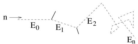
Fig. 6.8. A series of neutron–nucleus elastic scatters leading to the thermalization of the neutron.
