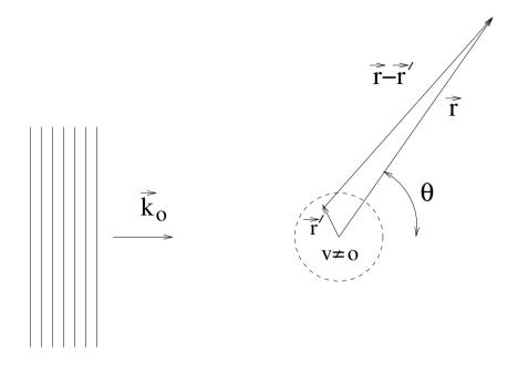
Fig. 3.16. A wave packet of central momentum  $p_0 = \hbar k_0$  that impinges upon a region with  $V(r) \neq 0$ . The scattered wave packet at r is the superposition of spherical waves generated at each point r'. A particle observed at r will be interpreted as having a momentum  $p' = p_0 r/r$  implying a momentum transfer squared of  $|q|^2 = |p' - p|^2 = 2p_0^2(1 - \cos\theta)$ .
