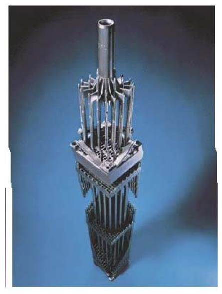
**Fig. 6.9.** Fuel element holder for a PWR reactor. The figure shows the control rods in place. When filled, the structure contains 264 zirconium tubes of length  $4\,\mathrm{m}$  and diameter  $9.5\,\mathrm{mm}$  containing pellets of  $\mathrm{UO}_2$ .
