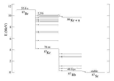
**Fig. 6.13.** Decay diagram of <sup>87</sup>Br. 2.3% of the β-decays are to excited states of <sup>87</sup>Kr that have excitation energies greater than the neutron separation energy of <sup>87</sup>Kr,  $S_n = 5.518 \,\mathrm{MeV}$ . These states decay by neutron emission.
