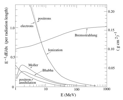
Fig. 5.11. Energy loss of electrons and of positrons in lead as a function of the incident energy [1]. The left scale uses the radiation length of lead (0.56 cm) as the unit of length. Ionization dominates at low energies while bremsstrahlung dominates above 10 MeV. Subdominant contributions come from wide-angle elastic scattering on electrons (*Moller* for electrons and *Bhabba* for positrons) and positron annihilation.
