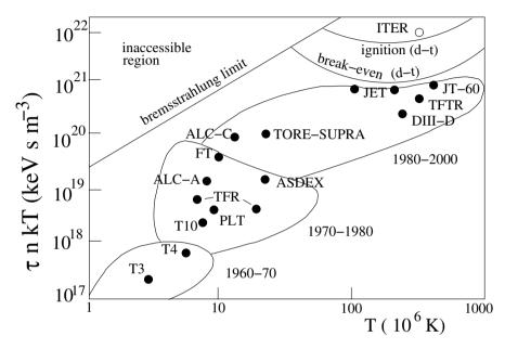
Fig. 7.7. Performance of various Tokamaks. The ITER project is projected to start construction in 2005. Above bremsstrahlung limit, cooling by radiation limits the temperature (Exercise 7.6).
