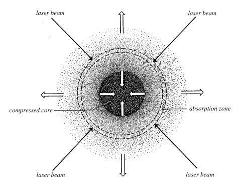
**Fig. 7.9.** Sketch of laser induced fusion. The d-t sphere interacts with the laser beams and it is vaporized superficially. By reaction, the corona compresses the central core.
