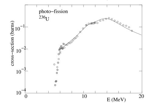
Fig. 6.5. Cross-section for  $\gamma^{236}U \rightarrow fission$  [30].
