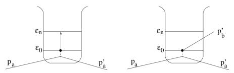
**Fig. 3.18.** Scattering of particle a on particle b in a bound state. Particle b can be left in bound state (left) or ejected from the potential (right).
