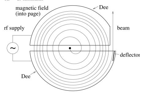
Fig. B.5. Schematic of a cyclotron. Particles are injected near the center of a dipole magnetic field and then spiral outward as they gain energy each time they pass through the alternating electric field between two electrodes called "Dee's." The radio-frequency is tuned to the particle's cyclotron frequency,  $\omega_c = qB/m$ . Near the maximum radius, the particles are deflected out of the cyclotron.
