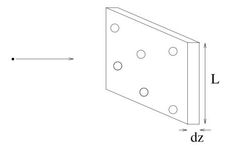
Fig. 3.1. A small particle incident on a slice of matter containing N=6 target spheres of radius R. If the point of impact on the slice is random, the probability dP of it hitting a target particle is  $dP = N\pi R^2/L^2 = \sigma n dz$  where the number density of scatterers is  $n = N/(L^2 dz)$  and the cross section per sphere is  $\sigma = \pi R^2$ .
