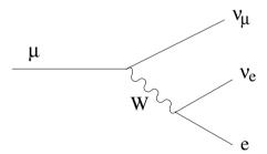
Fig. 4.22. Decay process of the muon.
