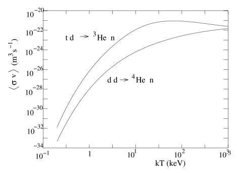
**Fig. 7.4.** Variation of the pair reaction rate  $\langle v\sigma \rangle$  as a function of the temperature for d-d and d-t mixtures.
