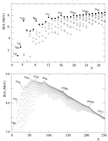
Fig. 1.2. Binding energy per nucleon, B(A,Z)/A, as a function of A. The upper panel is a zoom of the low-A region. The filled circles correspond to nuclei that are not β-radioactive (generally the lightest nuclei for a given A). The unfilled circles are unstable (radioactive) nuclei that generally β-decay to the lightest nuclei for a given A.
