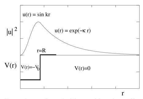
**Fig. 1.10.** A square-well potential and the square of the wavefunction  $\psi(r) = u(r)/r$ . The depth and width of the well are chosen to reproduce the binding energy and radius of the deuteron. Note that the wavefunction extends far beyond the effective range of the s=1 nucleon–nucleon potential.
