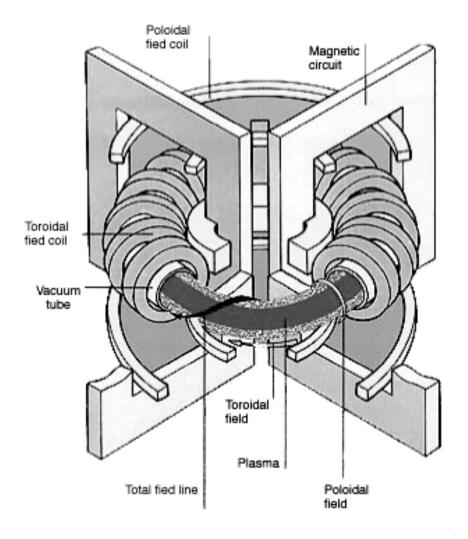
Fig. 7.5. Diagram of a Tokamak.
