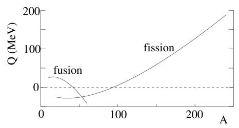
Fig. 6.1. The energy release in fission and self-fusion as predicted by the Bethe-Weizsäcker formula (2.13) for β-stable nuclei. Only nuclei with 40 < A < 95 are stable against both fission and self-fusion. In this figure,  $Q_{\rm fis}(A,Z)$  is calculated for symmetric fission,  $A_1 = A_2 = A/2$  and  $Z_1 = Z_2 = Z/2$ .  $Q_{\rm fus}(A,Z)$  is calculated for the production of a single nucleus of A' = 2A and Z' = 2Z.
