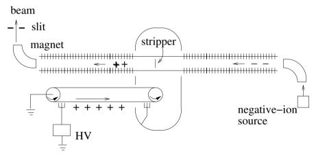
**Fig. B.2.** A schematic of a tandem Van de Graff accelerator. Negative ions are accelerated to the positive potential where a "stripper" removes electrons. The resulting positive ions are then accelerating to ground potential where a definite charge state is selected by a magnetic field and slit.
