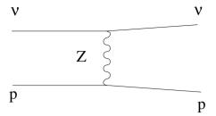
Fig. 4.30. Neutrino-proton elastic scattering mediated by the exchange of the  $Z^0$ boson.
