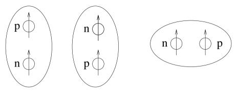
Fig. 1.11. The tensor potential for the s=1 state (1.59) makes the configuration on the right  $(\boldsymbol{\sigma} \cdot \boldsymbol{r} = 0)$  have a different potential energy than the two configurations on the left  $(\boldsymbol{\sigma} \cdot \boldsymbol{r} \neq 0)$ . This results in the permanent quadrupole moment of the deuteron.
