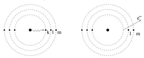
**Fig. 4.6.** An excited nucleus can transfer its energy to an atomic electron which is subsequently ejected from the atom. The process is called "internal conversion." The ejected electron can come from any of the atomic orbitals. In the figure, an electron from the deepest orbital is ejected, so-called K-conversion. Ejection of electrons in higher orbitals (L-, M-... conversion) are generally less probable.
