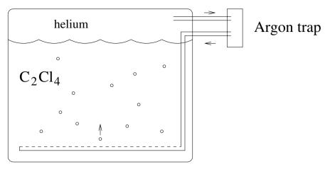
**Fig. 8.17.** The principle of the Homestake neutrino experiment.  $^{37}$ Ar atoms produced by neutrino absorption are swept out the the  $C_2Cl_4$  by bubbling helium gas through the liquid. The argon is then separated in a cold trap and introduced into a small proportional counter where the electron-capture decays of  $^{37}$ Ar are observed
